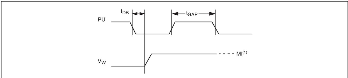
**Note:** (1) MI in the A.C. timing diagram refers to the minimum incremental change in the wiper voltage.
